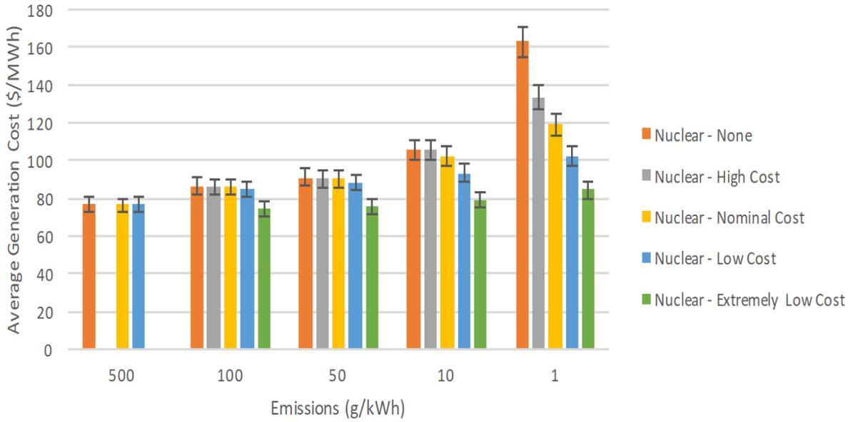
Figure 3.1.a: Texas Cost of Electricity Generation <sup>7</sup>
