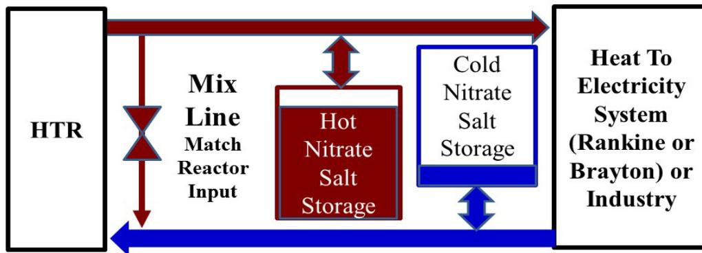
*Fig. D.4. Two-Tank Liquid-Salt Heat Storage*
