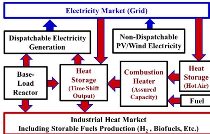
Fig. A.1. Nuclear Cogeneration System with Heat Storage
