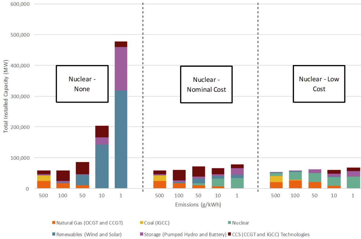
Figure 4.2.e: Optimal Capacity Mixes for United Kingdom
