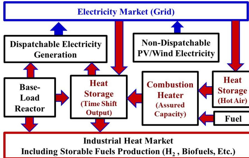
Fig. 7.1 Low-Carbon System Design
