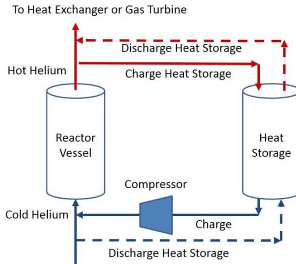
Fig. D.1. HTGR with At-Pressure Heat Storage
