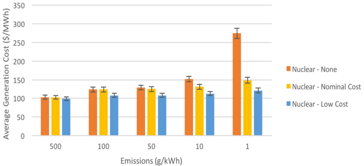
Figure 3.1.f: France Cost of Electricity Generation<sup>5</sup>
