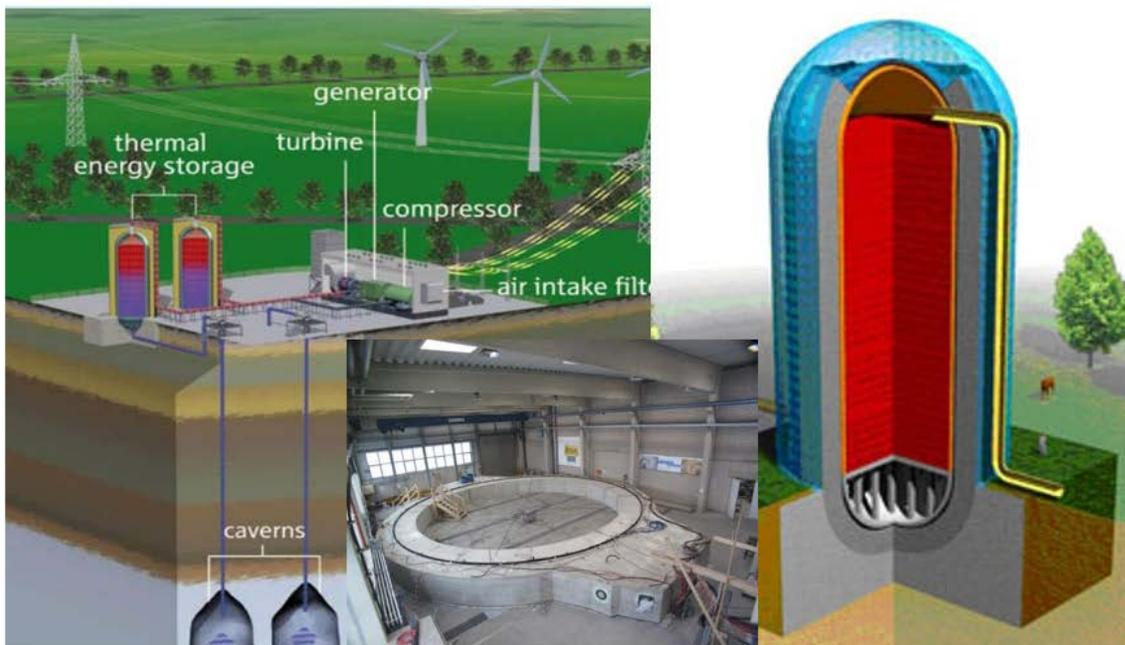
*Fig. D.3. Project Adele system, laboratory section of prestressed pressure vessel and schematic of the pressure vessel. Courtesy of General Electric, RWE AG, and Zublin.*
