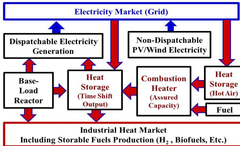
Fig. S. 6. Integration of Electricity, Industrial and Storable Fuels Energy Sectors with Heat Storage
