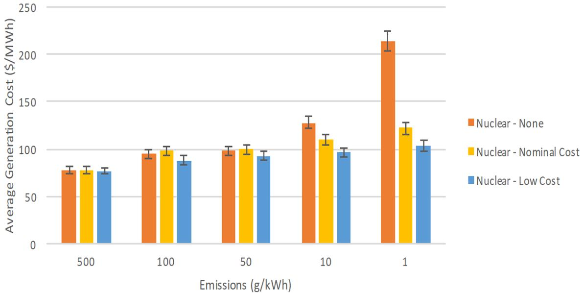
Figure 3.1.b: New England Cost of Electricity Generation <sup>5</sup>
