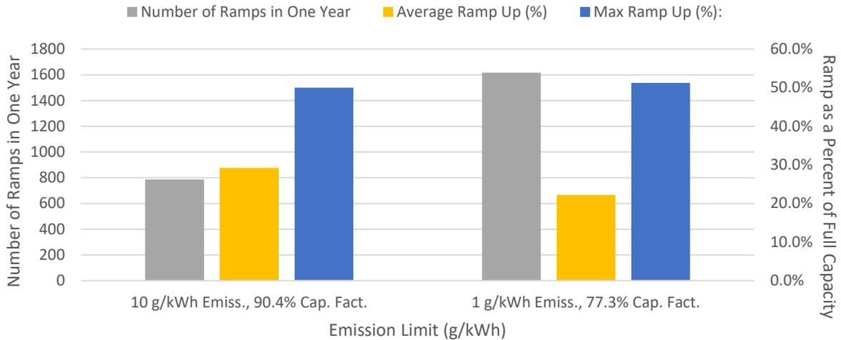
Fig. S.3. Texas ERCOT Nuclear Operations for Different Carbon Constraints
