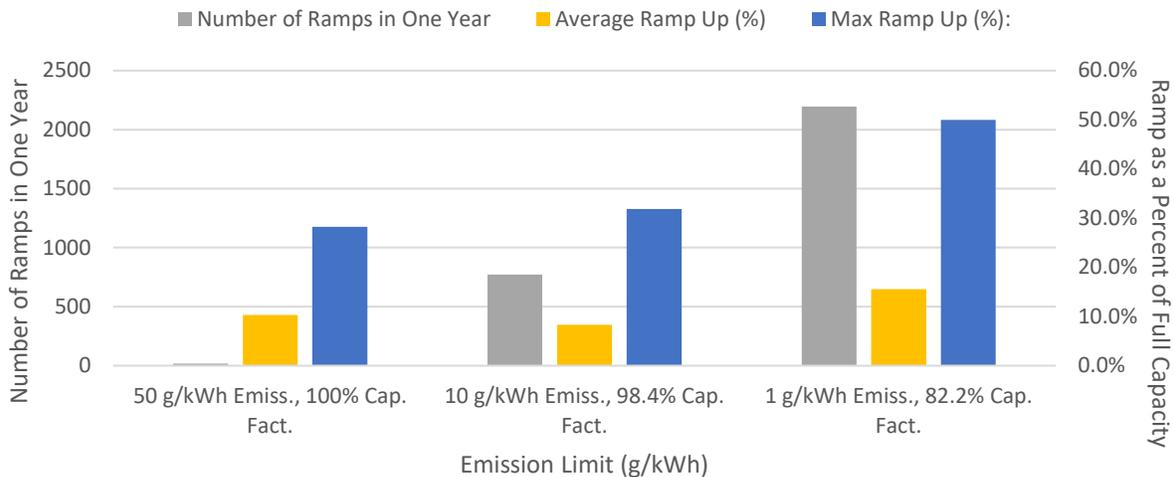
Figure 6.3.b: New England Nuclear Power Ramping
